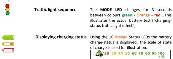
The voltage of the battery can be read through the 10 orange Status LEDs of SkyFire LCU. If all 10 LEDs light up, the battery is fully charged (charge-status scale: 100%).
