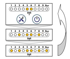
To enable the monitoring of the reception quality (RQO), the **FailSafe mode** of the lighting channel of the receiver must be activated! As signal level for the FailSafe Mode, the "smallest" possible Level ( $<950\mu s$ ) or the "highest" possible Level ( $>2100\mu s$ ) shall be programmed in the transceiver.
