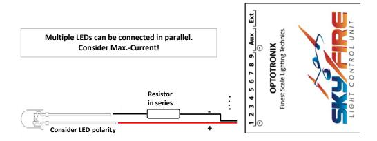
Only connect LEDs to the **SkyFire LCU**, **if the outputs have been programmed.** This prevents fusing of the LEDs which might have only been designed for flash mode (possible higher current) at an output which is still programmed to continuous light.
