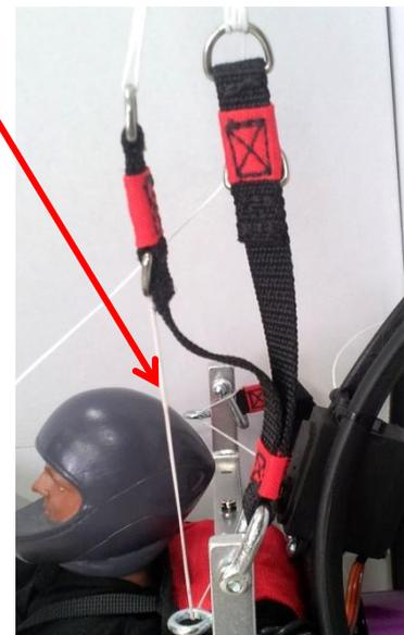
*Using the accelerator the A lines are shortened by a servo. The angle of the para is flatter so it can reach higher speed. Not accelerated the risers (A lines) have their full length. To accelerate the servo turns clockwise and pulls the lines.*
