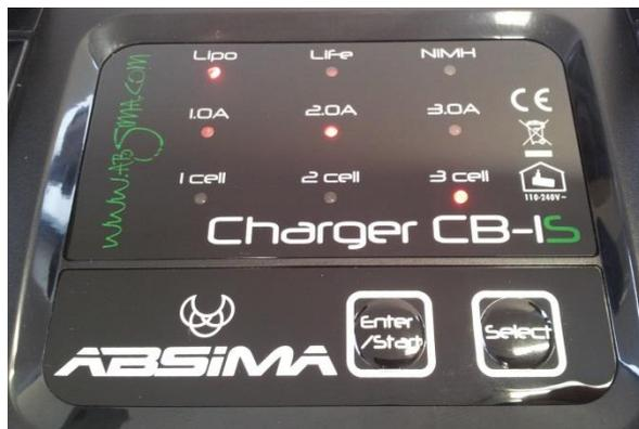
*Plug in the charger to 230V and adjust the parameters for the battery. By pressing the “Select” button for a long time you can select the parameter. By pressing the “Enter” button the value can be changed. Please select “LiPo – 2.0A – 3 cell” as shown in the picture.*
