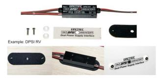
Now feed both screws through the mounting holes. The screws serves as positioning helps for the self adhesive cellular rubber strip which itself serves as protection against vibration. It is pushed over both screws from the inside and is fixed to the inner side of the fuselage. The anti-vibration mat is not mandatory but straightens out little bumps in the fuselage's side wall.
