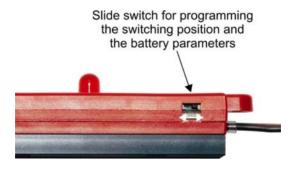
Programming is accompanied and controlled by different indications of the central LED in the RCS (RV). There are two "functional groups" to be programmed for the **DPSI Micro - RCS (RV).** One group refers to the servo signal, the other to the current supply:
