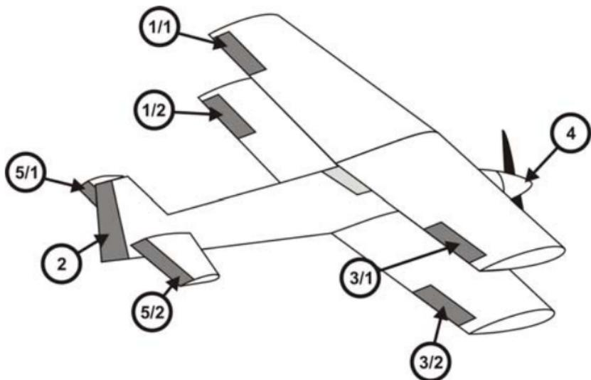
A biplane with 4 aileron servos, split elevator- and one yaw-rudder servo. The throttle servo may be directly connected to the receiver as an option.
