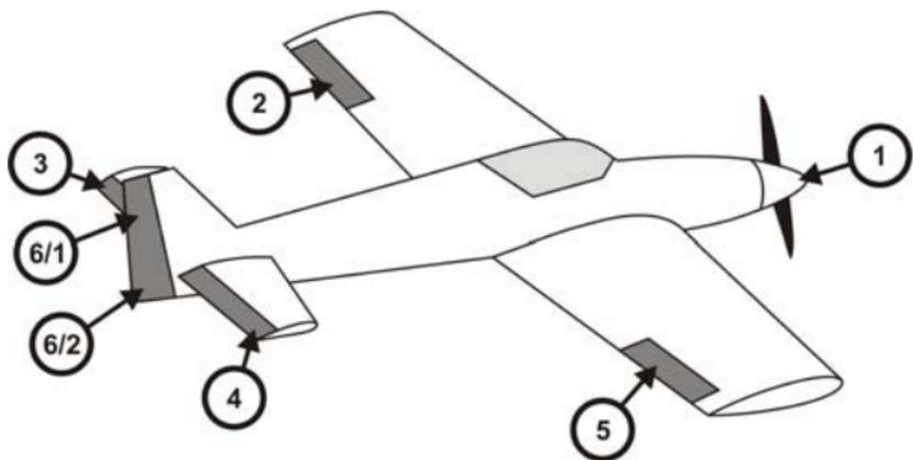
An acrobatic airplane with one servo per rudder, the yaw rudder is actuated by 2 servos.
