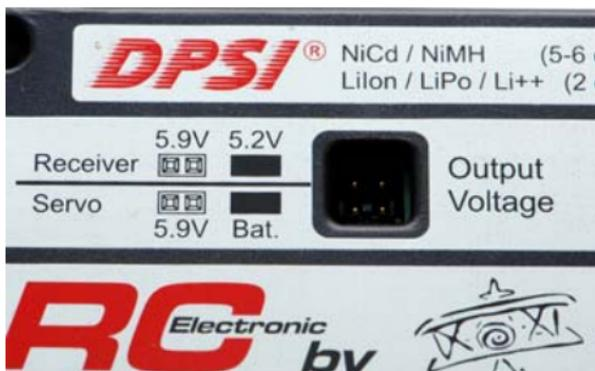
Selecting full battery voltage for the servos (receiver stays at 5.9V):
