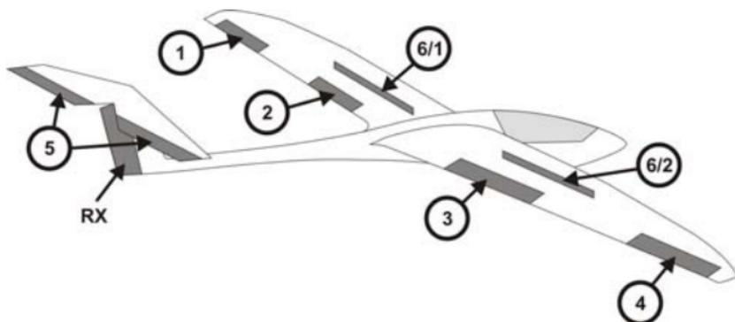
A glider with flaps and spoilers. The yaw rudder (and if so one tow release) are directly connected to the receiver.
