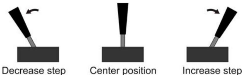
If the stick remains in one end-position, steps automatically increment or decrement after 2.5 seconds. This serves for quicker settings of the values.
