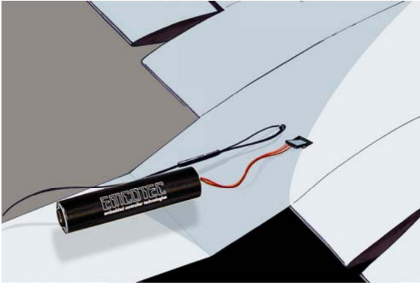
After the tow rope releases, the plug of the Locating Beeper slides out of its socket; the Locating Beeper sounds the S.O.S. alarm signal. If the rope falls into a field it is easily localized due to the alarm signal of the Locating Beeper. Connecting the shorting jumper stops the alarm (see 4.2.).
