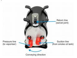
Flow direction is marked by an arrow. The "R" marked connector (swing fixture) is to be routed back to the tank. Back flow is approx. 35ml/min. In order not to install a separate connector to the tank, a delivered T-piece can be looped into the tanking hose. Here, the back flow is to be connected.
