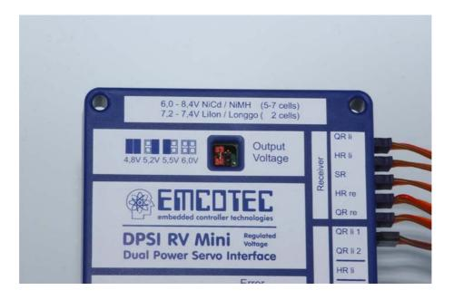
The jumper position is printed on the housing of each DPSI RV.
