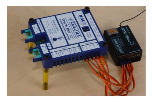
As a general rule, your must always ensure that the fastening is as vibration-free as possible and has sufficient air circulation. Reduction of vibration is particularly important for the receiver, since it reacts far more sensitively to mechanical vibrations than the "DPSI RV / RV Mini".
