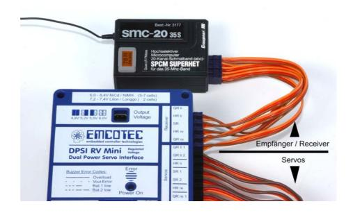
If two receivers are to be used, this is likewise feasible. The connection cables desired in each case are then connected to the receiver at which they are needed. Two receivers on the DPSI RV:
