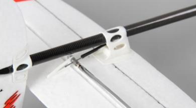
Screw the elevator on to the fuselage with the plastic screw. Then slide the rod into the ring, and tighten the screw to fix the wire at the elevator-rudder.
