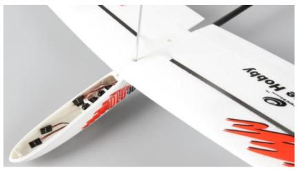
Slide the servo-cable of the wing through the opening in the fuselage forward in direction of the canopy.
