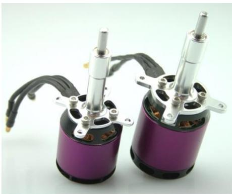
*Now slide the adapter over the shaft and fix it with the four included screws. Fasten the screws once all are screwed in. The bearing of the adapter must be in axial alignment to the bearings of the motor. This can be checked by removing and mounting again the bell. The shaft must slide in the bearings without any noticeable resistance.*
